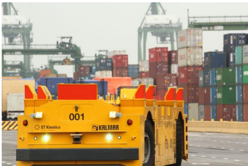
Figure 6: Automated Guided Vehicle in action (Source: Business Times Singapore)
