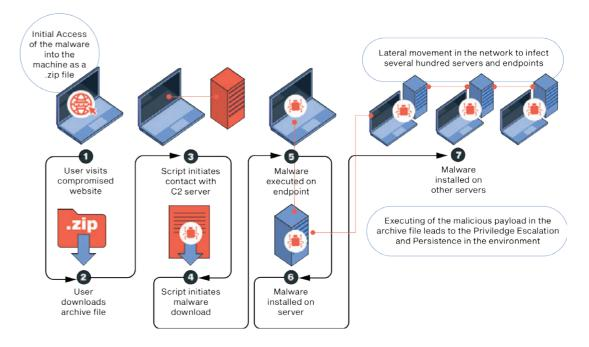
Figure 3: Schematic diagram of the attack campaign
