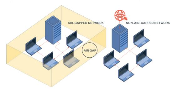
Figure 1: Graphical representation of an "air-gapped" system which is used in many OT environments. Such systems are not directly connected to the internet. Data can only be passed to it physically (e.g. via USB or removable media with another machine).
